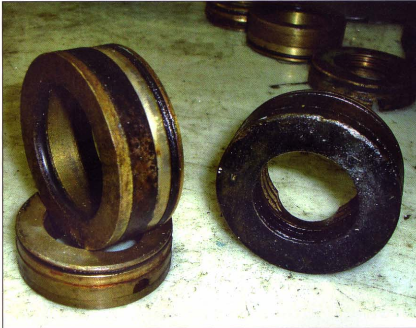
Fig. 3. Despite 20 years of 24/7 service, these Inpro/Seal bearing isolators were found to be working flawlessly—even though the pumps they protected had worn out.
