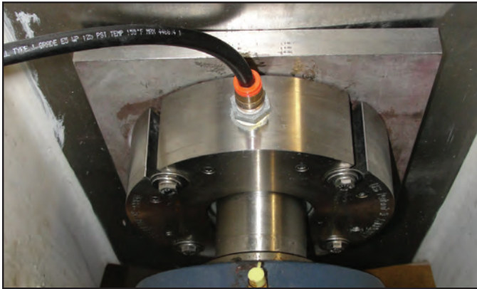
The stainless steel food grade Inpro/Seal Air Mizer is a permanent shaft sealing solution that meets all FDA requirements.
